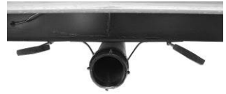
Black/Grey tank drain & valves
